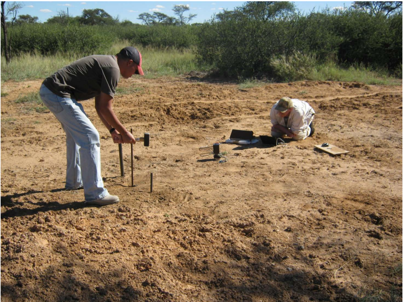
The above photograph, figure 1, shows the percussion, geophone, 'electronic box' and mini field computer
